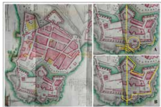
Fig. 6 – Ajaccio: an overpopulated small town (F. M. Accinelli, Storia...cit ). The castle fills up almost half of urban area. It was built by adapting a theoretic typology (A) to the geomorphological conditions (B).
