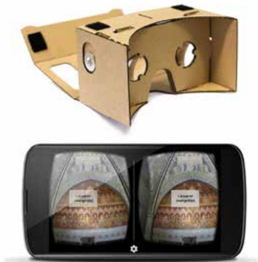
Fig. 6. The stereoscopic viewing of the application inside your smartphone for a vision properly with Google Cardboard.
