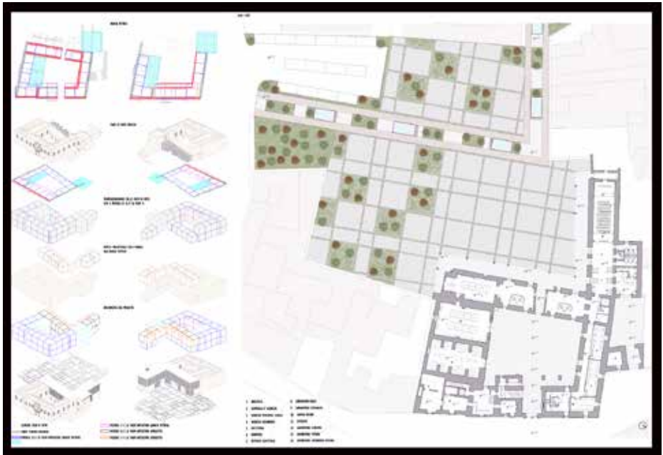
Fig.8 Domenico Nardi, School of Design project for the reuse of Palazzo Vernazza: the 26x26 Palmi Napoletani module re-draws the outer space of the garden, the new volumes, and, subdivided into a pattern of sub-modules re-draws the horizontal and vertical surfaces in an isomorphic.
