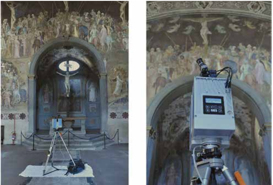
Fig. 2. Survey with laser scanner Phase-Shift Z+F Imager 5006h and acquisition of colour with camera.
