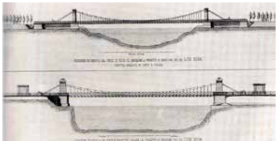
Fig. 6a This bridge, consisting of two spans of 85 m. each, linking Tournon-sur-Rhône to Tain-l'Hermitage, put into service on 25/8/1825, was actually the first large suspension bridge in continental Europe. The bridge, suspended by eight iron cables, has a total length of 170 m. [Cotte, 1986]. Fig. 6b Elevation and plan of the bridge on the Garigliano (1832), Luigi Giura design (1826); see: Di un nuovo ponte sospeso a catene di ferro sul Garigliano in Annali Civili del Regno delle Due Sicilie T. 1. Napoli: Dalla Tipografia del Real Ministero degli Affari Interni, 1833; p. 41-51 (span length: 80.40 m.s.; wide deck: 5.50 m.) .
