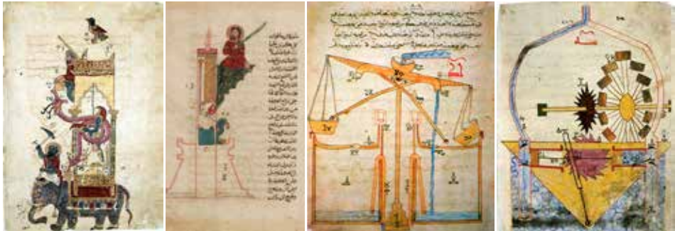
Fig. 1a al-Jazarī's elephant clock. Fig. 1b al-Jazarī's candle clocks. Fig. 1c al-Jazarī's hydropowered perpetual flute. Fig. 1d al-Jazarī's reciprocating pump, from The Book of Knowledge of Ingenious Mechanical Devices [al-Jazarī, 1974].
