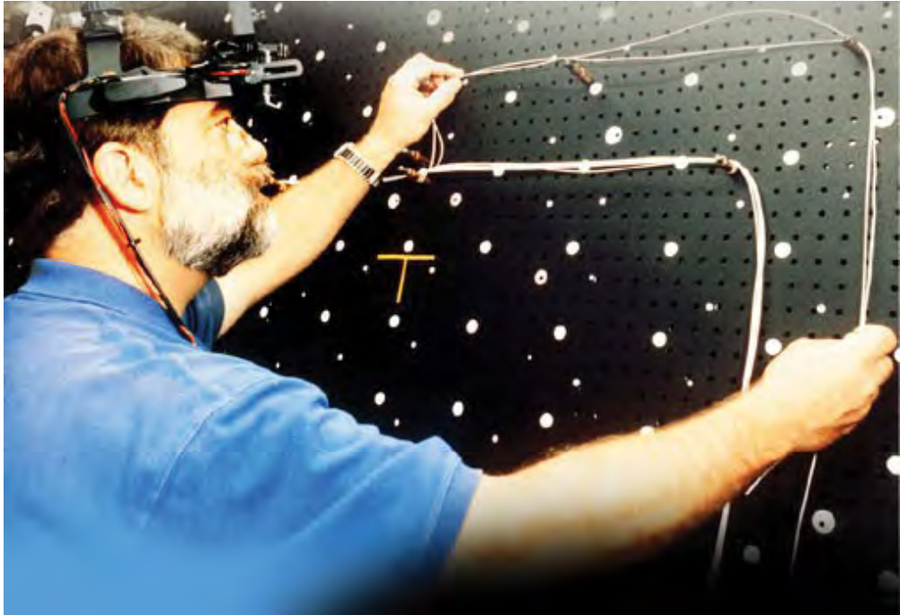
Fig. 1: Researchers at Boeing used a see-through HMD to guide the assembly of wire bundles for aircraft. Image of
