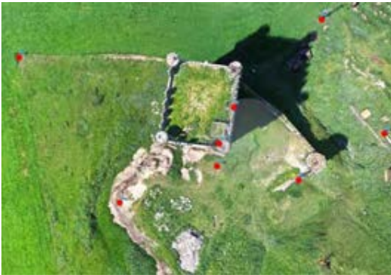
Fig. 3 Location of control points around the castle. Figure 4 Control Points or targets.
