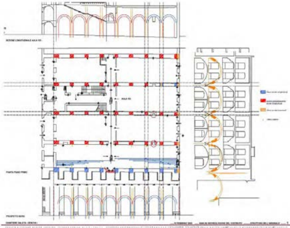
Fig. 4 The "arches-and-pillars structure detected during restoration yard in early 2000s.
