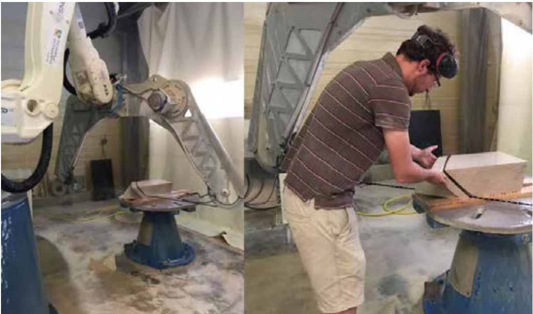
Fig.13 Prototype realized with the diamond wire cutting technique moved by an anthropomorphic robot
