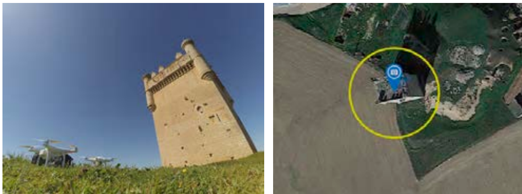
Fig. 5 and 6 Photographic RPAs next to the tower of the castle of Belmonte de Campos (Palencia), Orbital Flight Program of the RPA on the tower.
