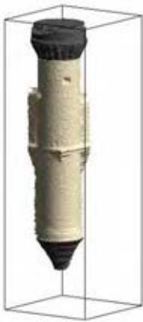
Figure 17 Moderated tower gatehouse with PointSense for Heritage imported to Revit.
