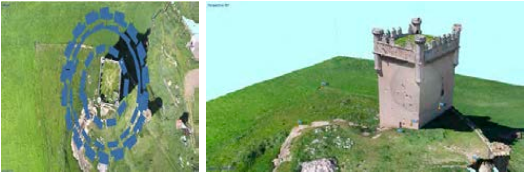
Fig. 8 Frames taken with the RPA and oriented in the Agisoft PhotoScan. Figure 9 Point cloud obtained by photogrammetry in PhotoScan
