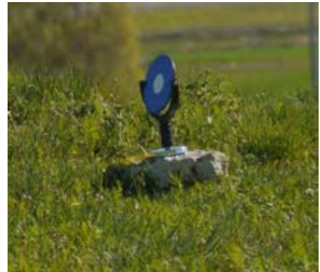
Fig. 3 Location of control points around the castle. Figure 4 Control Points or targets.
